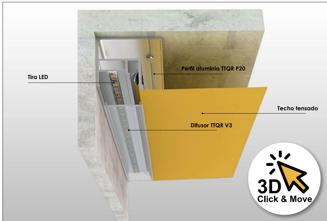
EL SISTEMA TTQR CROWN LIGHT SE COMPONE DE PERFIL DE ALUMINIO TTQR P20, TIRA LED Y DIFUSOR TTQR V3
